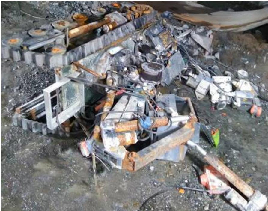
*An Army robot was recovered at 944 metres. This Wheelbarrow Revolution Mk8 robot was sent into the drift before the second explosion as part of operations at that time.*
