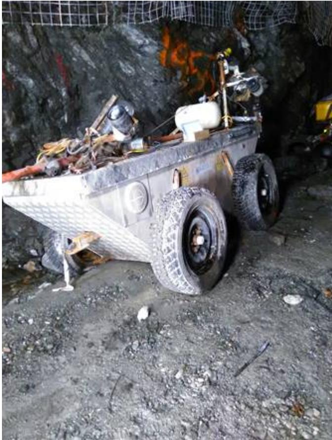
*A Water Corporation robot was recovered at 953 metres. The robot measures 1.3 metres high by 1.0 metre wide by 2.4 metres long. It weighs about 1,200 kg. This robot carried another smaller robot which travelled further up the drift as far as Russell Smith's loader at 1,560 metres and should be recovered from there.*
