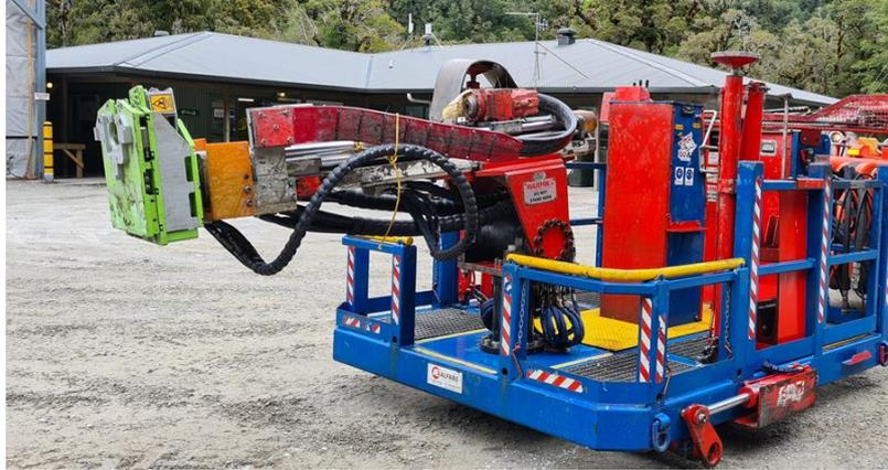
*A "lobster" attachment (the green bit) on the front of a drill rig at the Pike River Mine site*
