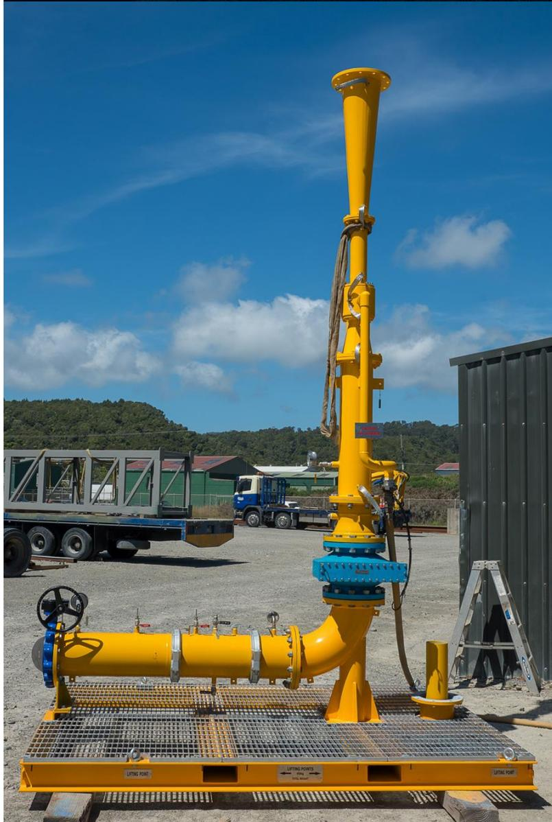
*This venturi will sit atop new borehole 53 and works like a vacuum cleaner to draw gases from the mine drift. It is due to be installed in the next few days.*
